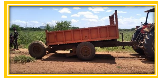
Broken axel which fell off of trailer.
